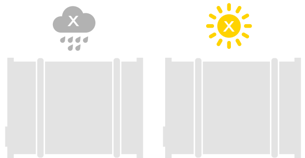
FIGURE 3: Storage position: unexposed to weather, drums on side and raised off the ground
