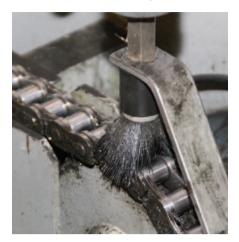
Transmission chains can be found throughout a bottling plant, activating internal parts of machines and driving conveying systems. These chains require continous lubrication to reduce friction and wear, noise, higher energy consumption and, of course, unplanned production stops.
