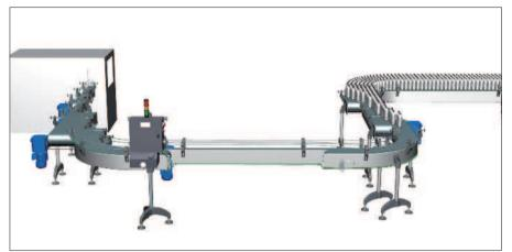
Flat-top conveyor chains require constant lubrication to prevent high friction between packages and chains in accumulation areas. The typical solution is to apply high volumes of a water and soluble lubricant mixture, which can cause operator accidents due to slippery floors or package quality issues resulting from organic development and moisture formation. The humid atmosphere can cause corrosion, which leads to replacement costs and reduced line efficiency.
